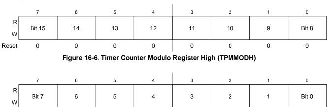
Figure 16-7. Timer Counter Modulo Register Low (TPMMODL)
