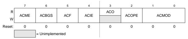
Figure 8-3. ACMP Status and Control Register
