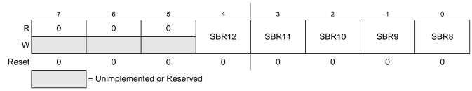
Figure 14-5. SCI Baud Rate Register (SCIBDH)
