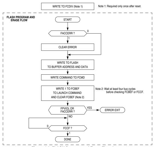
Figure 4-2. FLASH Program and Erase Flowchart
