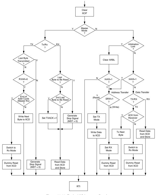
Figure 11-11. Typical IIC Interrupt Routine
