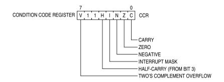
Figure 7-2. Condition Code Register
