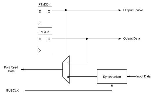
Figure 6-1. Parallel I/O Block Diagram
