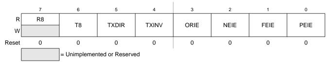
Figure 14-11. SCI Control Register 3 (SCIC3)
