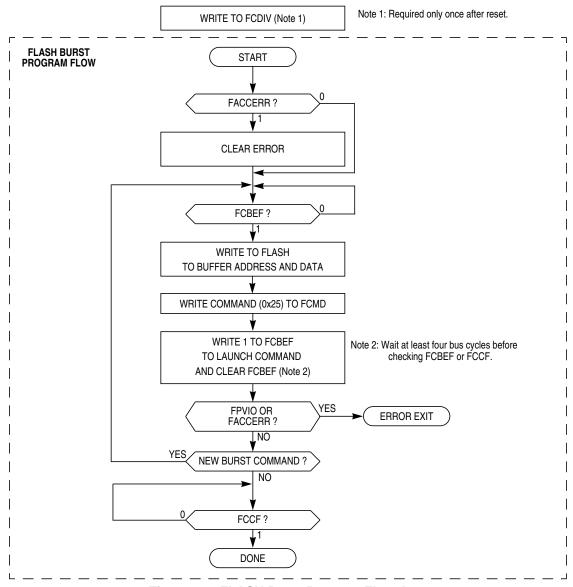
Figure 4-3. FLASH Burst Program Flowchart
