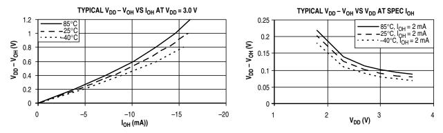
Figure A-4. Typical High-Side (Source) Characteristics — Low Drive (PTxDSn = 0)
