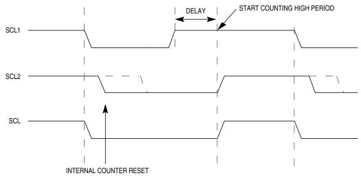
Figure 11-9. IIC Clock Synchronization
