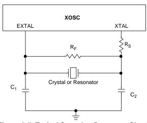
Figure A-7. Typical Crystal or Resonator Circuit
