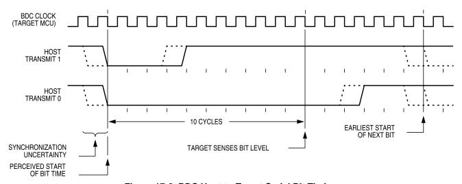
Figure 17-2. BDC Host-to-Target Serial Bit Timing
