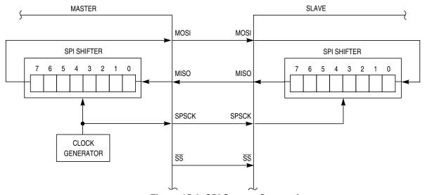
Figure 15-2. SPI System Connections
