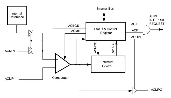
Figure 8-2. Analog Comparator (ACMP) Block Diagram
