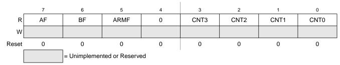
Figure 17-9. Debug Status Register (DBGS)
