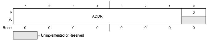
Figure 11-3. IIC Address Register (IICA)
