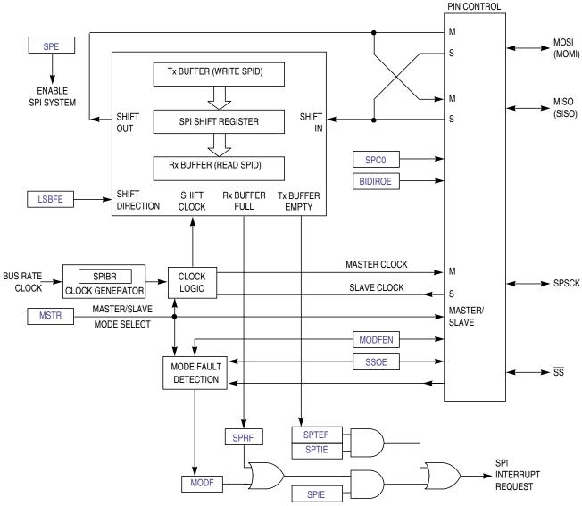
Figure 15-3. SPI Module Block Diagram
