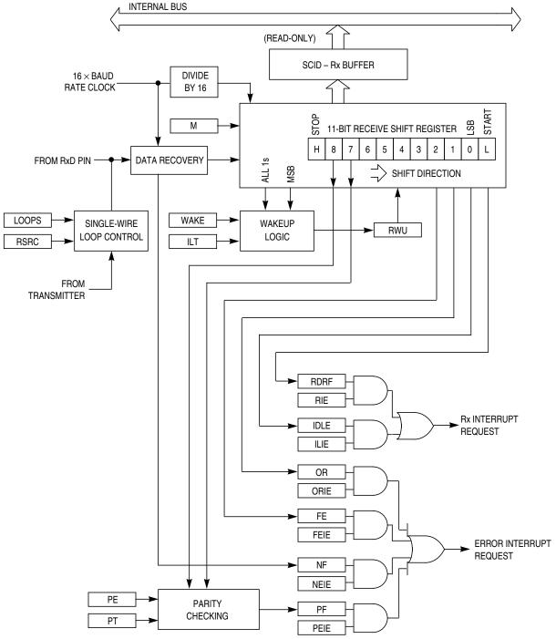
Figure 14-4. SCI Receiver Block Diagram
