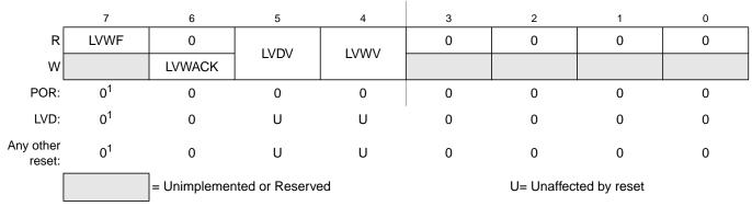
Figure 5-12. System Power Management Status and Control 3 Register (SPMSC3)
