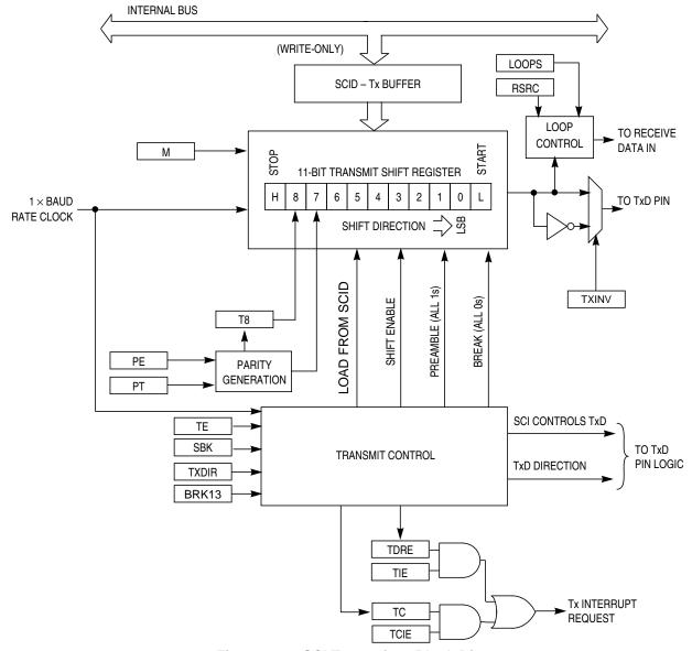
Figure 14-3. SCI Transmitter Block Diagram
