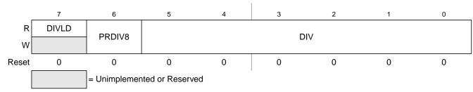
Figure 4-5. FLASH Clock Divider Register (FCDIV)
