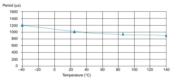
Figure A-8. Typical RTI Clock Period vs. Temperature
