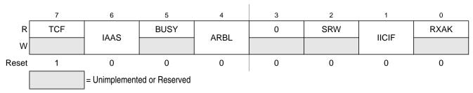
Figure 11-6. IIC Status Register (IICS)
