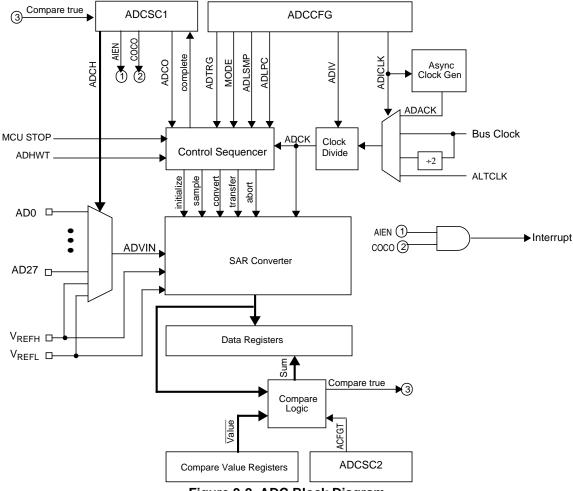
Figure 9-2. ADC Block Diagram
