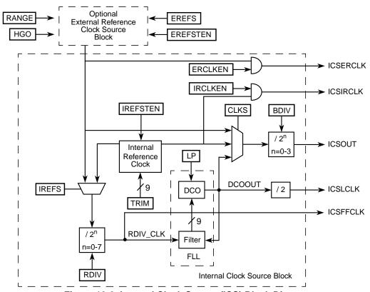
Figure 10-2. Internal Clock Source (ICS) Block Diagram
