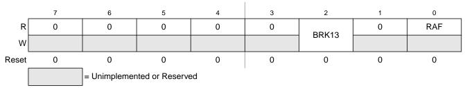
Figure 14-10. SCI Status Register 2 (SCIS2)
