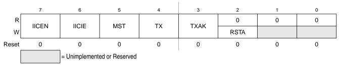
Figure 11-5. IIC Control Register (IICC)
