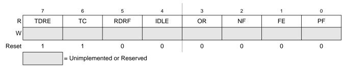
Figure 14-9. SCI Status Register 1 (SCIS1)
