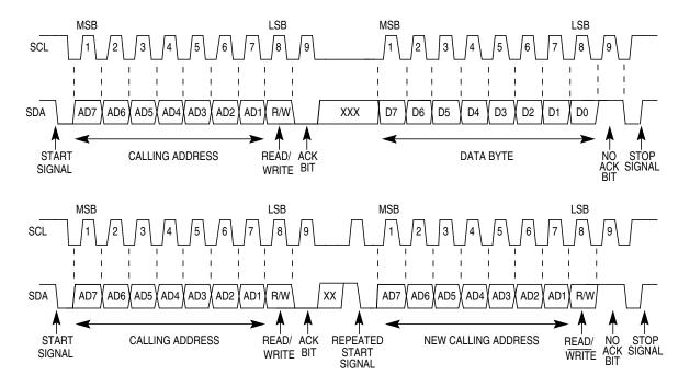
Figure 11-8. IIC Bus Transmission Signals
