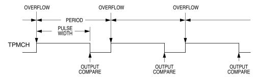
Figure 16-11. PWM Period and Pulse Width (ELSnA = 0)
