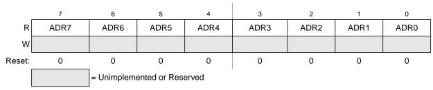
Figure 9-7. Data Result Low Register (ADCRL)
