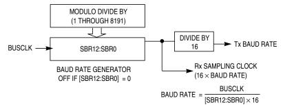
Figure 14-13. SCI Baud Rate Generation
