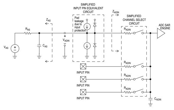
Figure A-17. ADC Input Impedance Equivalency Diagram
