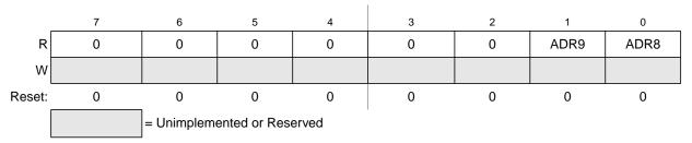
Figure 9-6. Data Result High Register (ADCRH)
