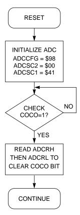
Figure 9-14. Initialization Flowchart for Example
