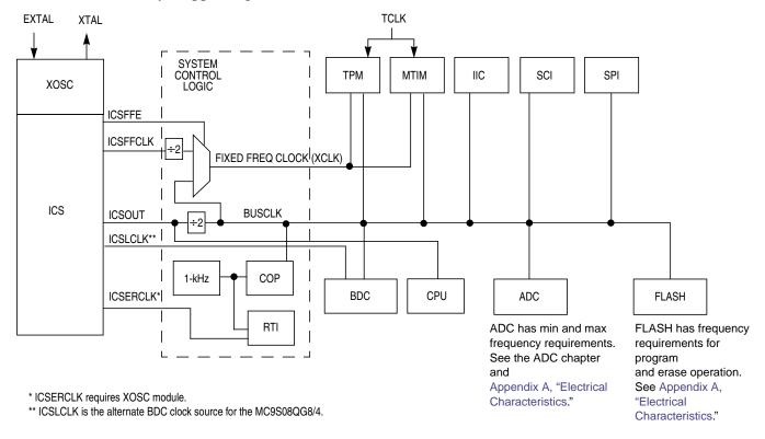
Figure 1-2. System Clock Distribution Diagram
