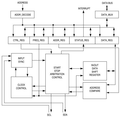
Figure 11-2. IIC Functional Block Diagram
