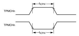
Figure A-12. Timer Input Capture Pulse
