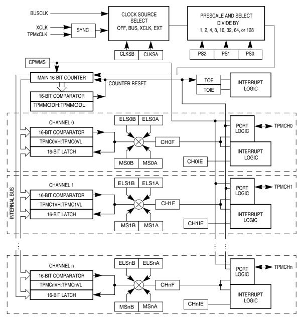
Figure 16-2. TPM Block Diagram
