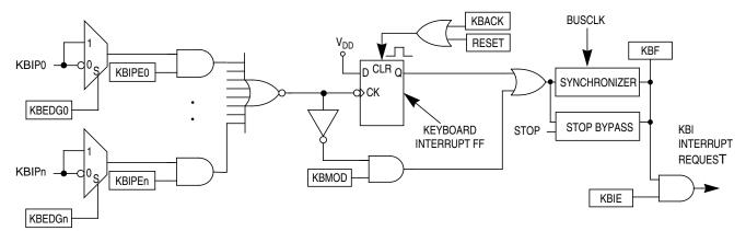
Figure 12-2. KBI Block Diagram
