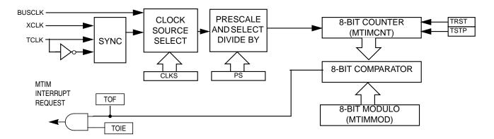
Figure 13-2. Modulo Timer (MTIM) Block Diagram
